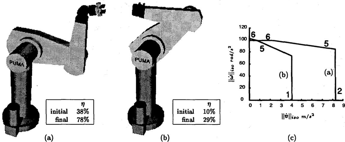
**Figure 7: PUMA 560 Actuation Efficiencies and Motion Isotropy Curves.**
