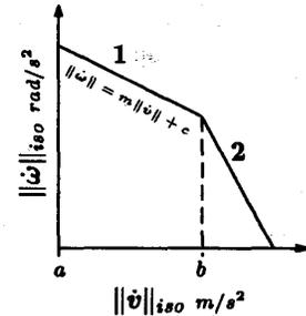
Figure 5: Motion Isotropy Curve.  $a$  and  $b$  values, and the equation for the first line segment of the curve.
