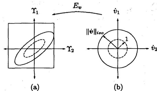
**Figure 1: 2 DOF Isotropic Acceleration.** The isotropic acceleration circle is mapped into a torque ellipse which is expanded/contracted until it touches the bounds.
