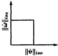
Figure 6: Isotropy Indicator. Rectangle suggests high degree of acceleration isotropy.
