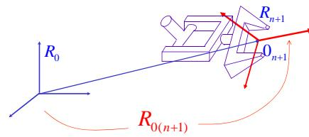
$$R_{0(n+1)} = \begin{pmatrix} r_{11} & r_{12} & r_{13} \\ r_{21} & r_{22} & r_{23} \\ r_{31} & r_{32} & r_{33} \end{pmatrix}$$
