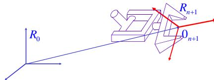
$$T_{0(n+1)}(q) = \begin{pmatrix} R_{o(n+1)}(q) & \rho_{o(n+1)}(q) \\ 0 & 1 \end{pmatrix}$$
